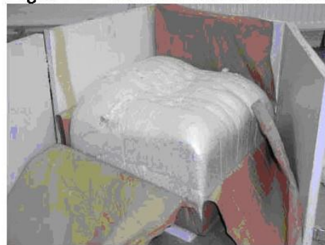
Figure 2: Cured foam in test box.
